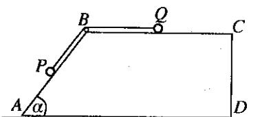
A light inextensible string of length  $l$  ( $> 2a$ ) passes over a small smooth pulley at  $B$ , and has a particle  $P$  of mass  $m$  attached to one end and another particle  $Q$  of the same mass  $m$  attached to the other end. The system is released from rest with the string taut, the particle  $P$  held at the mid-point of  $AB$  and the particle  $Q$  on  $BC$ , as shown in the figure.
