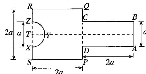
As shown in the adjoining figure, the lamina  $L$  is in equilibrium on a rough plane inclined at an angle  $\alpha$  to the horizontal with its plane vertical and the edge  $PS$  on a line of greatest slope such that the point  $P$  lies below  $S$ . Show that  $\tan \alpha < (2 - k)$  and  $\mu \geq \tan \alpha$ , where  $\mu$  is the coefficient of friction between the lamina and the inclined plane.
