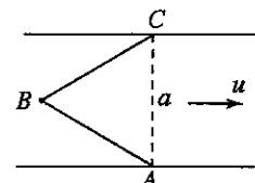
Show that the speed of the boat in its motion from  $A$  to  $B$  is  $\frac{1}{2}(\sqrt{4v^2 - u^2} - \sqrt{3}u)$  and find its speed in the motion from  $B$  to  $C$ .
