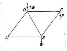
Draw a stress diagram using Bow's notation and hence, find the stresses in the rods stating whether they are tensions or thrusts.
